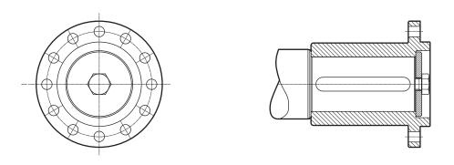
Thoroughly clean and degrease the flange of the gear unit and the area of the machine to which it is to be coupled. Safe torque transmission depends largely on the correct execution of this procedure. Do not use solvents or dirty rags to degrease mating surfaces.
