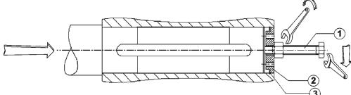
The tie bolt (1), spacer (2) and circlip (3) are not included in the supply.
