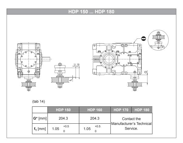
$L_0$  = Free height [mm] -  $L_1$  = Height under load [mm] -  $f_1$  = Deflection  $L_0$ - $L_1$  [mm] \* (nominal value)
