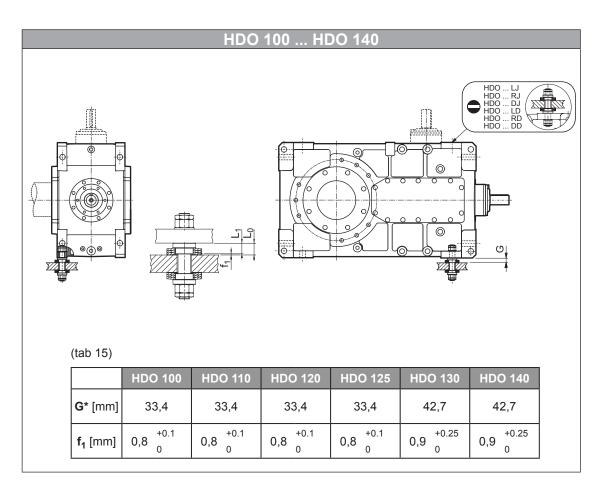
$L_0$  = Free height [mm] -  $L_1$  = Height under load [mm] -  $f_1$  = Deflection  $L_0$ - $L_1$  [mm] \* (nominal value)
