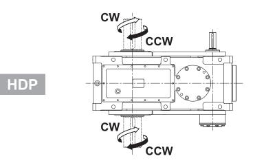
The backstop device is keyed to the end of the input shaft opposite the drive side in such a way that it is accessible for inspection and maintenance. The device shares the gear unit's own lubrication system.
