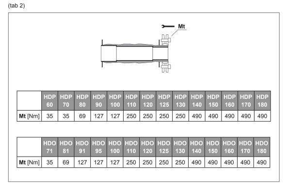
Torque the shrink disc as prescribed to assure axial fixing of the transmission, in the absence of external loads.
